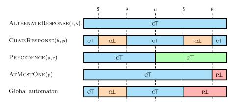
Fig. 13: Monitoring with local and global colored automata, showing a case where the global automaton detects a violation before it actually manifests on a single constraint.
